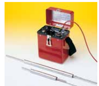
Model 1500 Linear Potentiometer pictured with Model RB-100 Readout Box.
