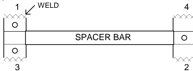
Figure 3 - Welding Sequence for the Mounting Blocks
