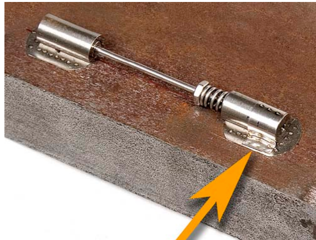
Figure 8 The Completed Collar Shim.
