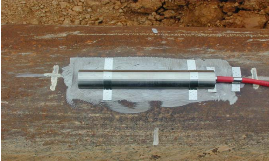
Figure 9 - Spot welded cover plate
