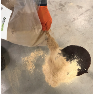
Step 1: Apply loose absorbent directly to the spill
