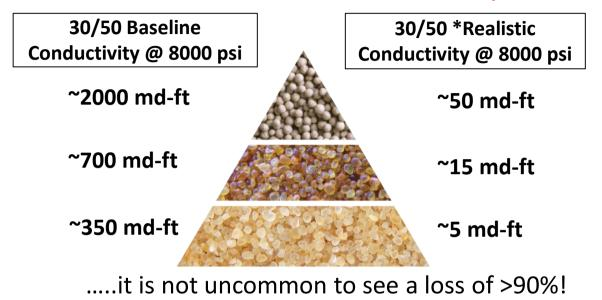
\*Tight Gas Condensate Reservoir Conditions Prop Conc. – 0.75 lb/sqft Frac Height – 200 ft Rate <u>per frac</u>: 300 mcfd, 100 BOPD, 1 bwpd Gel Damage, cyclic stress Temp – 275° F
